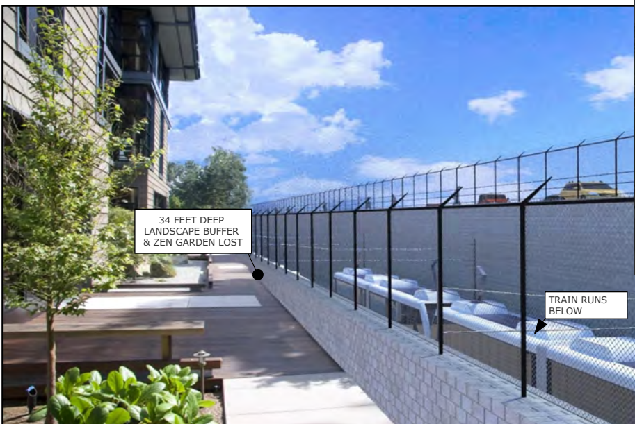
OPTION 4 RETAINED CUT/TRENCH CREATES 2 RETAINING WALLS TRAIN RUNS 20 FEET BELOW GRADE
